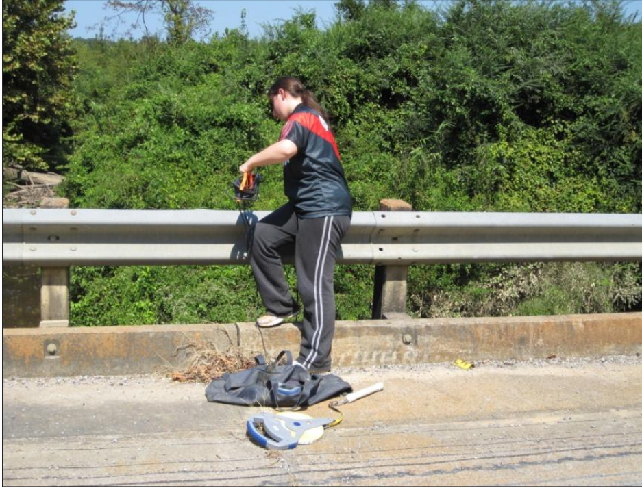
Figure 24 TROLL 9500 being deployed
