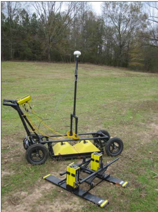
Figure 15 GPR system, 100MHz and 250MHz antennas, and DGPS
